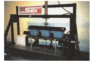
Static Load Test Set-Up
